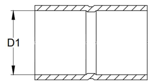
In the case of hydronic tubes and fittings, D1 = 0.627 In. This is because the inner diameter of the hydronic pipe is 0.500 In., and the coupling must consider the thickness of the wall. The result is: tube inner diameter + 2 x wall thickness + tiny gap for soldering/ brazing, pipe is 0.500 In., and the coupling has to take into account the thickness of the wall. The result is: tube inner diameter + 2 x wall thickness + tiny gap for soldering/brazing.
